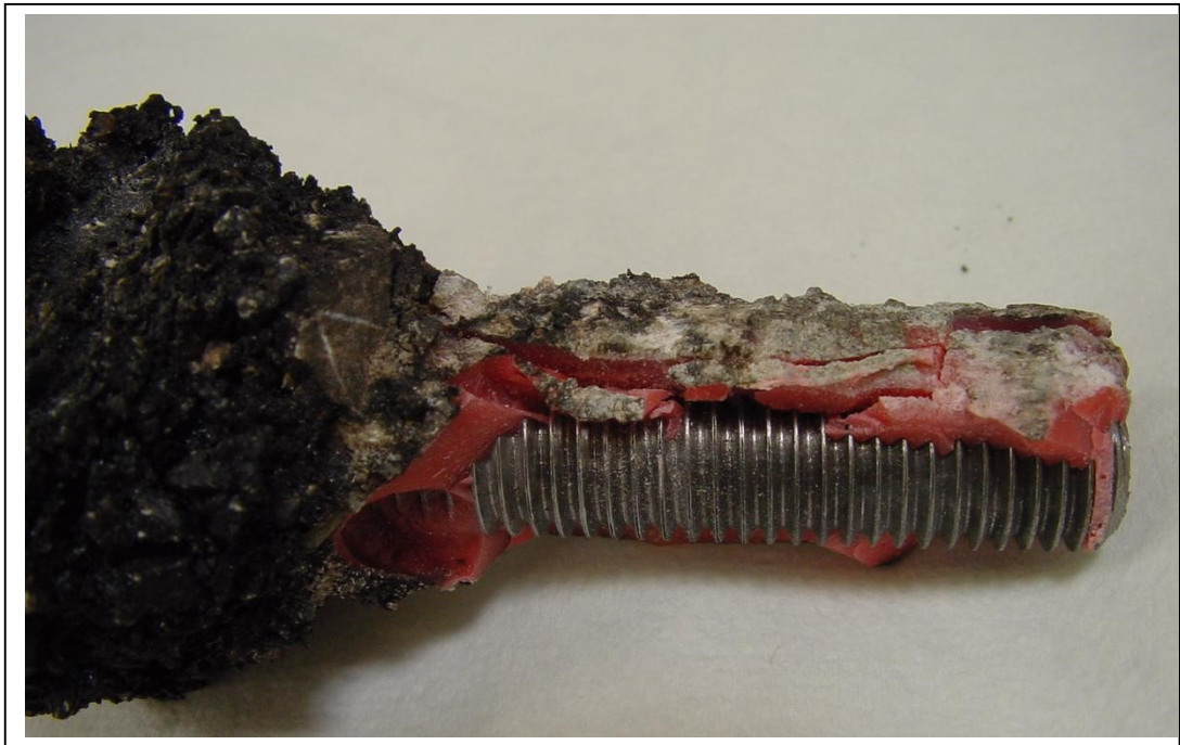
Fig. 4: The HIT-RE 500 injection adhesive is fully cured and bonded to the asphalt surrounding the adhesive.
