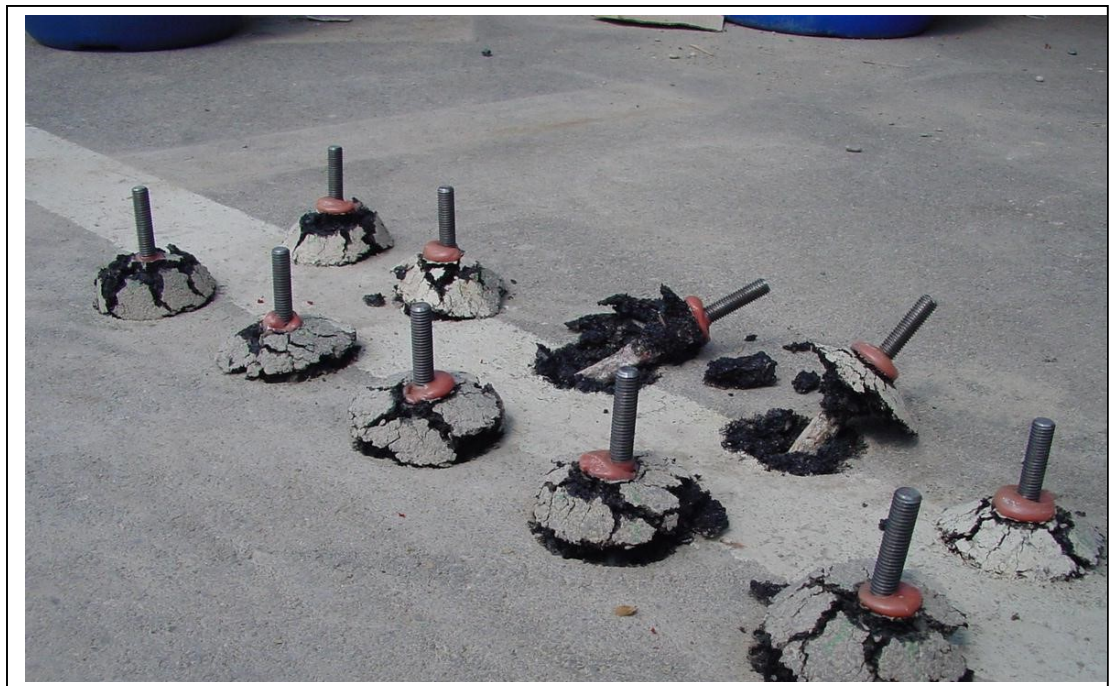
Fig. 2: Tensile testing of HAS M12 anchor rods fastened with Hilti HIT-RE 500 injection adhesive in asphalt base material. The failure mode of all anchors was breaking out of the asphalt.
