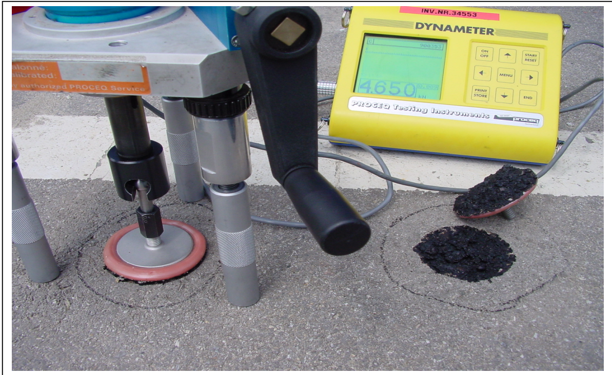
Fig. 5: Test arrangement for bonding test with HIT-RE 500 on asphalt; Test disc 50 mm / 2" in diameter
