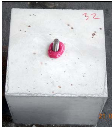
Specimen with installed anchor
