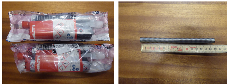
Figure 2. Injection mortar Hilti HIT-RE 500 V4 (left) and anchor rods M12x160 mm (right).
