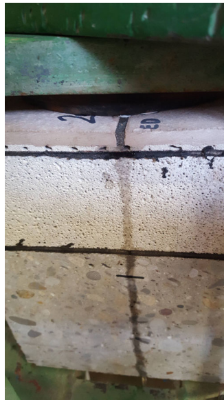
Figure 5. Escape of water during filling the testing apparatus with water.
