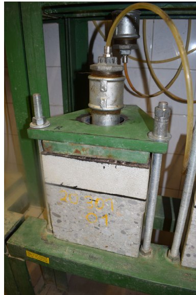
Figure 7. Specimen no. 20.301 01 after installing in the testing apparatus.
