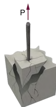
Fig. 2.11: Concrete cone breakout failure
