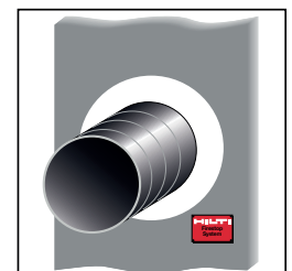
5. Fasten identification plate (if required)
