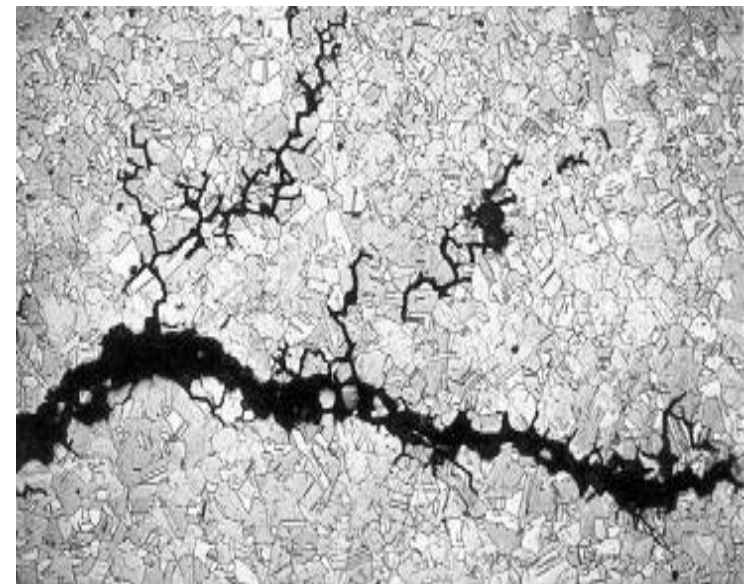
Accelerated crack propagation caused by corrosion and stress
