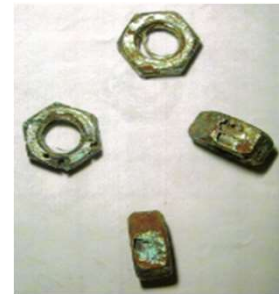
A4 nuts after 3 months coastal environment
