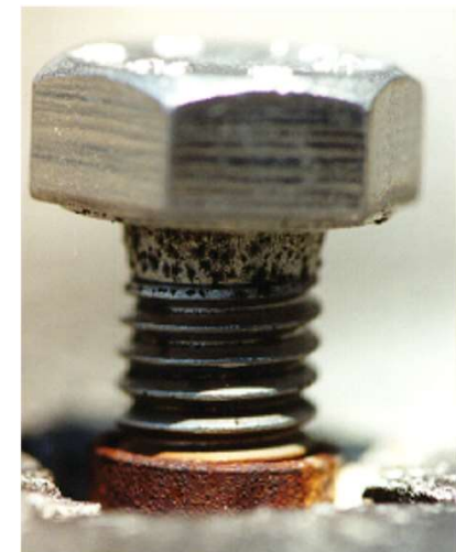
Galvanised HKD with an A2 bolt
