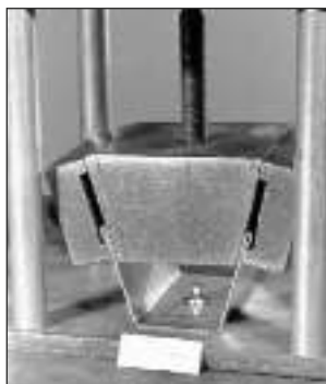
Pull-over test specimen at test start
