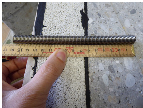
Figure 4. Definition of the borehole depth.
