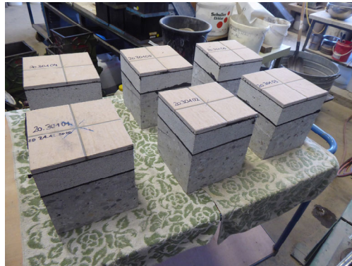
Figure 3. Composite specimens after wet cutting with dimensions of 200x200x235 mm.
