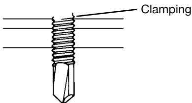
Thinner base material requires a coarser thread pitch to assure proper clamping. The thicker the material, the finer the threads must be. In very thick metal (3/8" to 1/2" thick), a fine thread is advisable. This will allow the thread to tap into the base material with less installation torque than a coarse thread.
