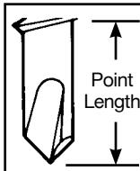
The unthreaded section from the point to the first thread should be long enough to assure the drilling action is complete before the first thread engages the drilled metal. Screw threads advance at a rate of up to ten times faster than the drill flute can remove metal. All drilling therefore should be complete before threads begin to form.
