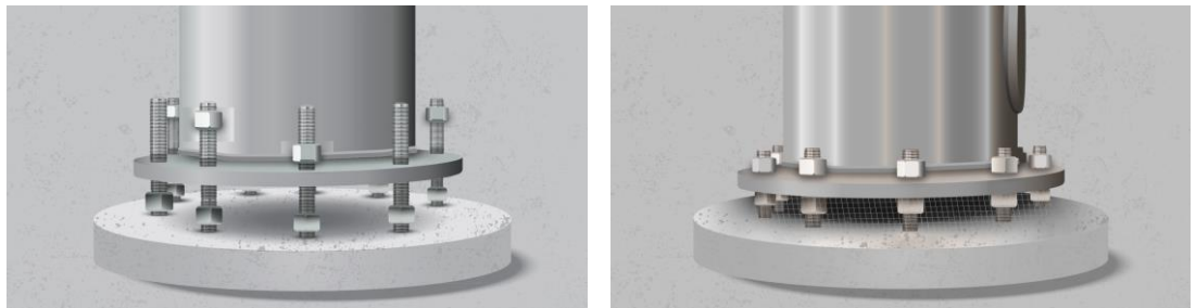
Figure 1. UngROUTED stand-off connection: during seating on leveling nuts (left) and in service (right)
