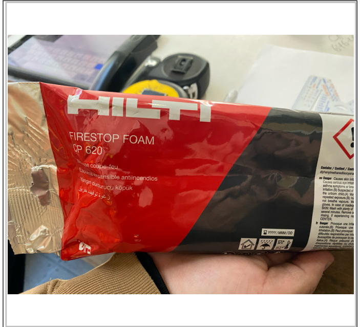
Hilti CP620 was used however, the material is tested for penetrating items, not for blank openings. The EJ is required.
