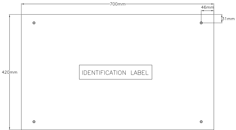
STAINLESS STEEL PROTECTION PLATE ELEVATION VIEW
