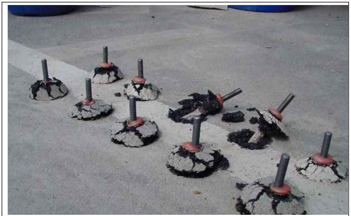
Picture 2: Tension test of anchors HAS M12 fastened with Hilti HIT-RE 500 injection mortar in base material asphalt. Failure mode for all anchors: asphalt failure
