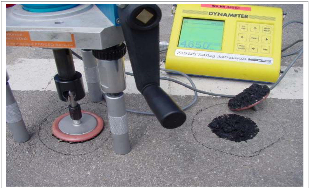
Picture 5: Test arrangement for bonding test of HIT-RE 500 on asphalt. Test discs with \varnothing 50\text{mm} / 2''
