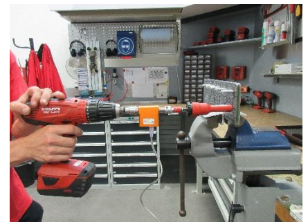
Test setup to test the forming torque of the studs in stainless steel base material
