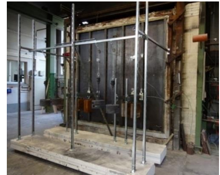
Figure 1: Test facility for fire test (big bulkhead)
