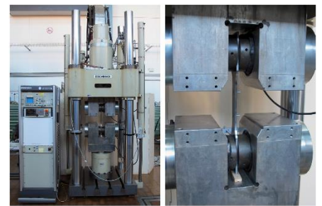
Test facility for fatigue tests
