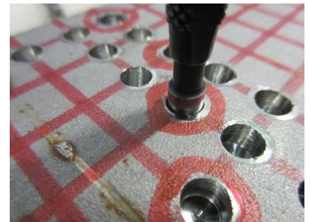
Testing of pilot hole quality
