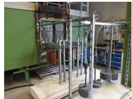
Figure 2: Test facility for fire test (small bulkhead)
