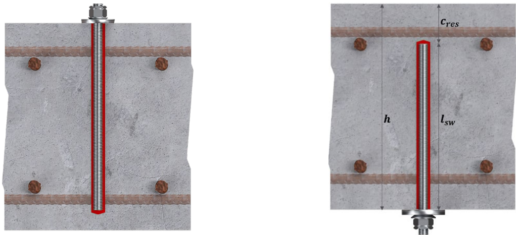
Figure 18: Simplified schematic of the HIT-Punching shear strengthening system installed from above (left) or below (right) the concrete member
