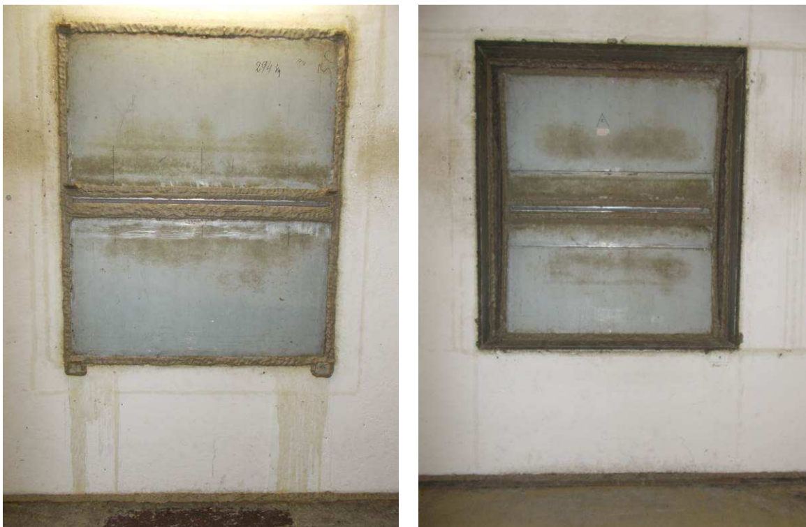
fig 3 Photos of the mounted element, taken by ift Laboratory for Building Acoustics
