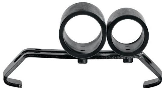
Check Gauge for HUS Screw Anchor Reusability Test
